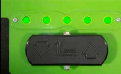
fig. 3B – Front Deck Motor Indicator Lights displaying green under normal operating conditions.
