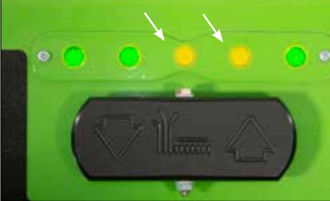
fig. 3C – Front Deck Motor Indicator Lights displaying yellow for blade 3 and 4 indicating tougher mowing conditions for those blades.
